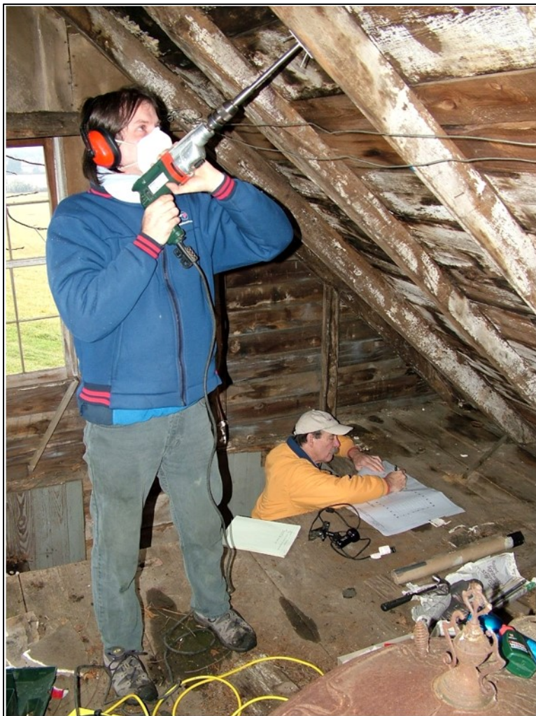
Figure 2. Michael Worthington of the Oxford Dendrochronological Laboratory taking a sample from a rafter for dendro-dating, while Professor Gary Stanton of the University of Mary Washington records the location.
