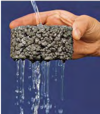
Porous Pavement: allows water to pass through, into a gravel bed.
