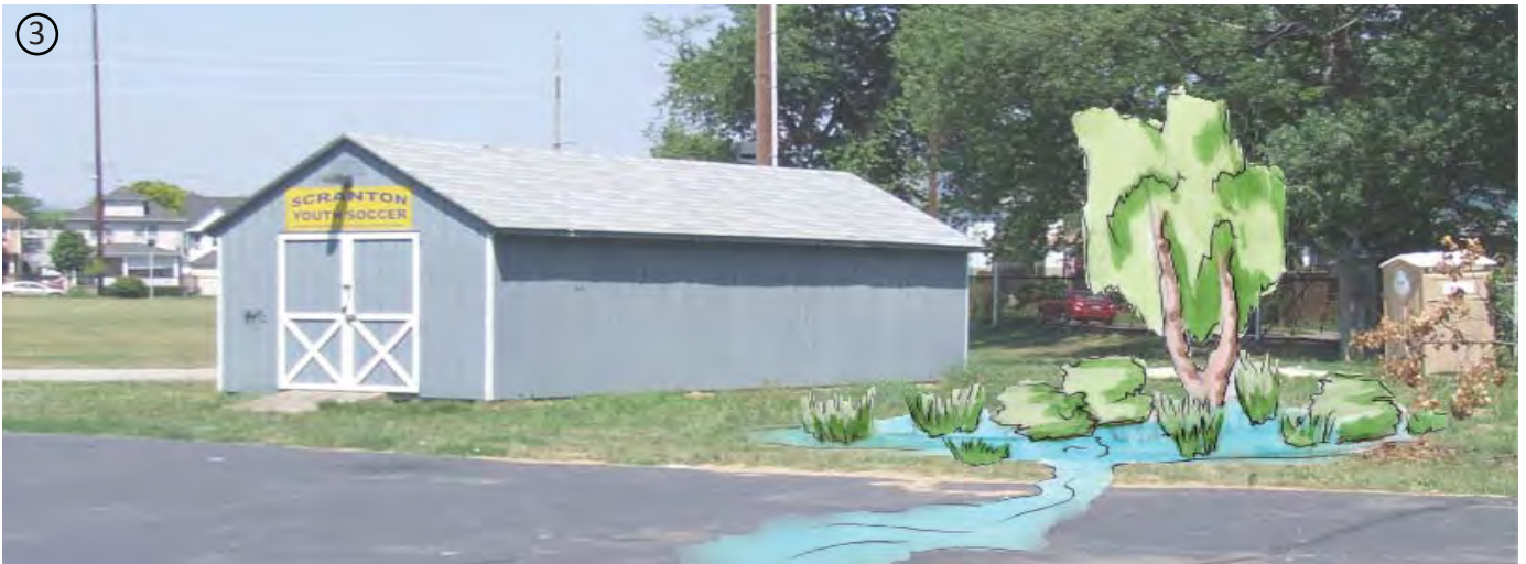
Mowed space next to the parking area can be converted into a rain garden to help filter runoff.
