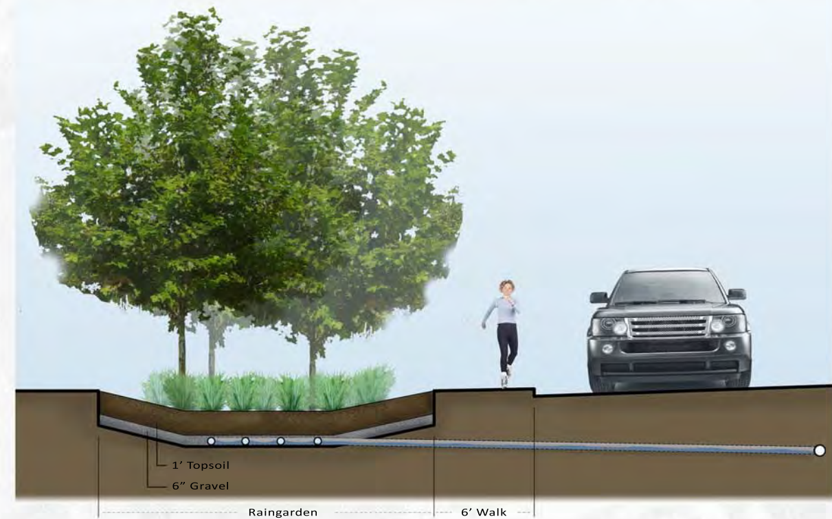
Raingarden With Underdrains
