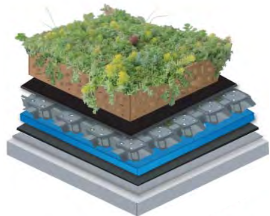
Diagram of an extensive roof with layers consisting of vegetation, growing media, filter fabric, drainage layer, root barrier and waterproofing membrane at the base.
