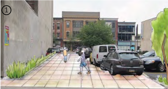
Proposed green alley that utilizes permeable pavers and underground storage to infiltrate water.
