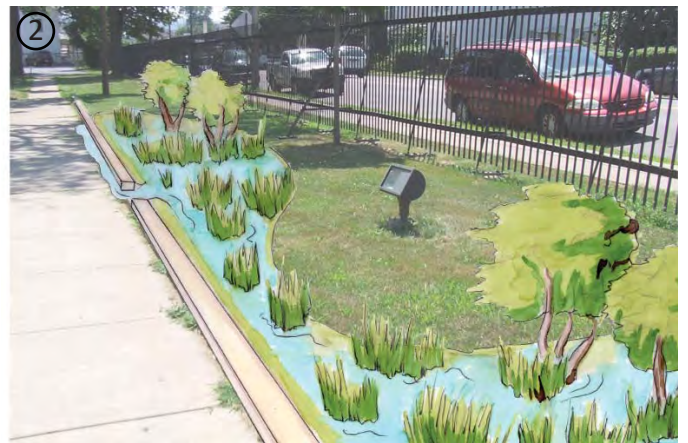
Curb cuts can be made to allow water to enter a series of connected rain gardens.
