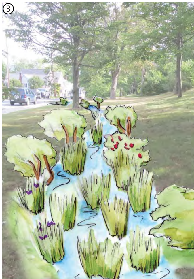
The swale would bring the water through the base of the park and allow any excess water to exit onto Webster Street.
