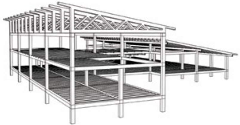
View of structural frame highlighting driven wood piles, glulam frame and wood trusses (Dobariya + Rissmiller)
