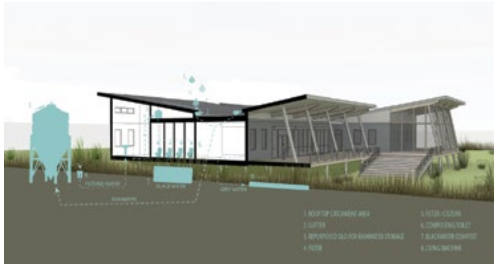
The roof form captures rainwater and stores it in the re-purposed silos. It is then filtered and treated using UV light and distributed back into the labs, bathroom and kitchen sinks, showers and toilets. The greywater from sinks and showers is piped into a living machine on the southwest side of the building that uses native plants to filter the water. (Robbs and Peters)
