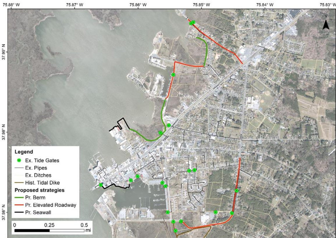
Figure 7. Concept-level structural strategies and tide gate locations.
