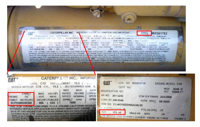
Caterpillar Nameplate (2 labels): EPA Family Name – 5CPXH0928EBK Engine Model Year - 2005 Engine Horsepower – 475 HP
