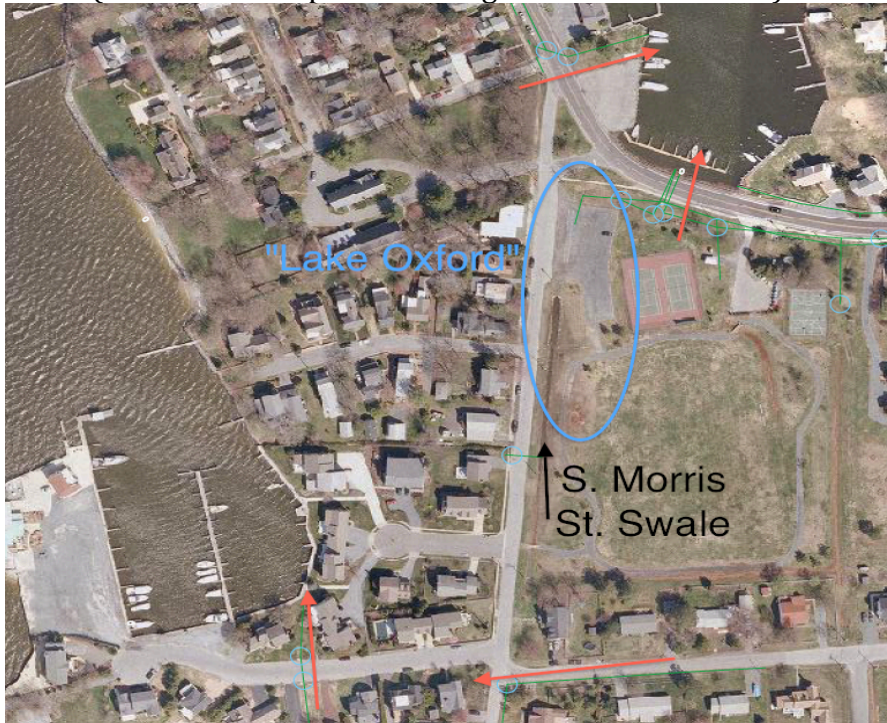
Map 4. South Morris Street area outfalls (in red), Lake Oxford (blue circle), and swale (as the dark strip inside along South Morris Street)
