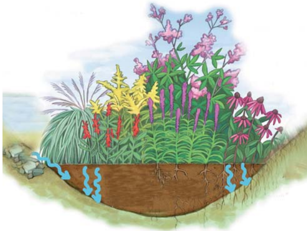
The plant roots within a rain garden help infiltrate water into the ground.
