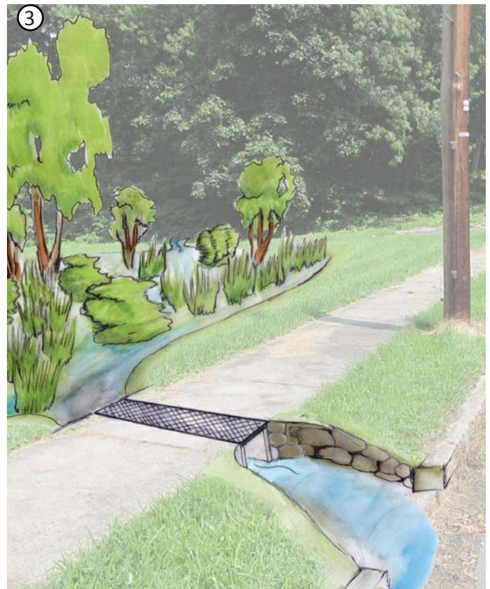
The existing curb can be cut with a pipe or trench drain extending under the sidewalk to allow water to enter the space.
