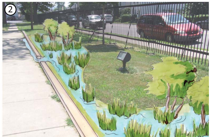
2 Curb cuts can be made to allow water to enter a series of connected rain gardens.
