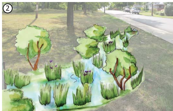
An inlet can be installed under a section of the walk toward the bottom of the park to allow street runoff to enter a vegetated swale within the park.
