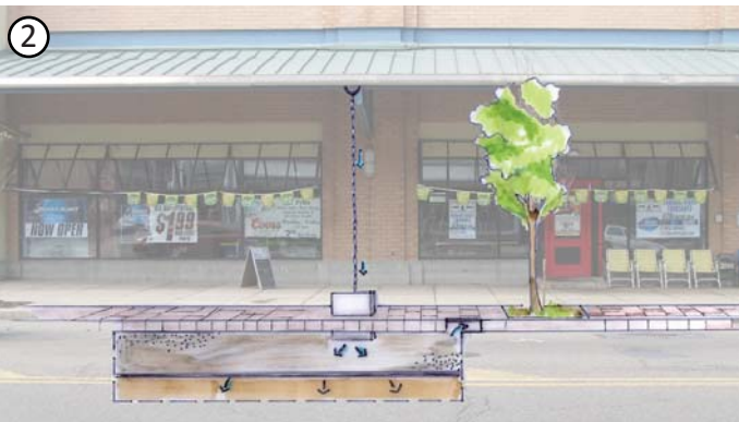
② The water can be brought into catchment containers and given the opportunity to infiltrate through underground storage.
