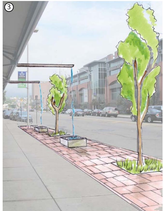
③ Even though storage units will be underground, the surface will be made of pervious pavers that do not take away from sidewalk space.
