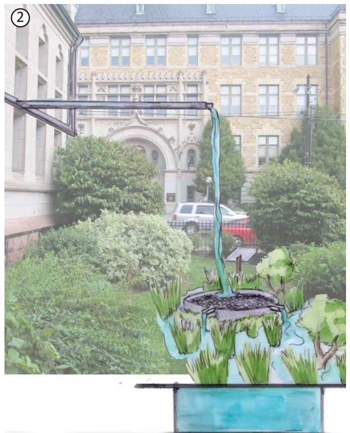
The mowed space behind the Albright Library will be retrofit with green infrastructure - artful downspout disconnect, educational signage, an underground cistern that over flows into a rain garden.
